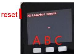
① Lidarbot- Long press C button and then press reset button (the red one) -----
