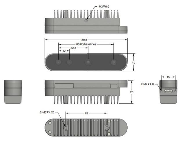
FIG 4 STRUCTURAL DRAWINGS
