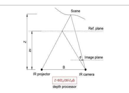
FIG 1 SCHEMATIC DIAGRAM OF THE MONOCULAR STRUCTURAL OPTICAL IMAGING PRINCIPLE
