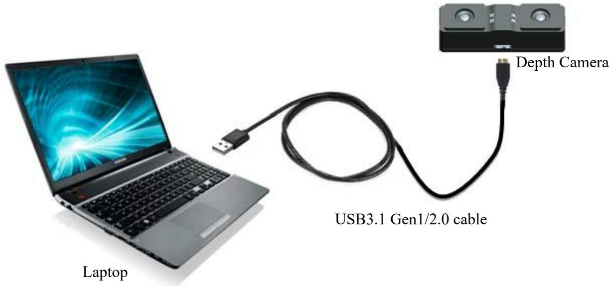
FIG 3-1. DEPTH CAMERA TO PC CONNECTION
