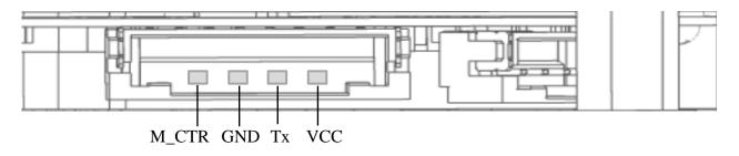
FIG 3 YDLIDAR X2 INTERFACES
