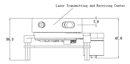
FIG 1 YDLIDAR X2 FRONT STRUCTURE SIZE (UNIT:MM)
