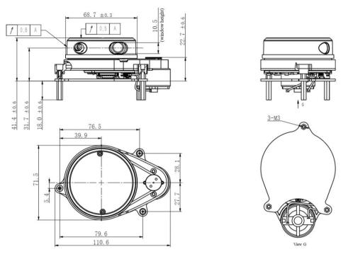
FIG 1 YDLIDAR X4PRO MECHANICAL DIMENSIONS (UNIT: MM)
