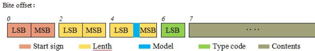
FIG 3 YDLIDAR TG Series SYSTEM MESSAGE DATA PROTOCOL
